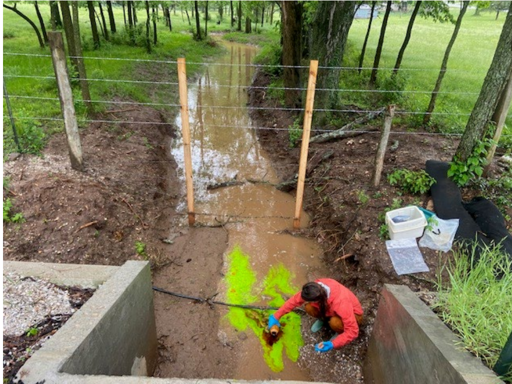
Figure 22. Fluorescein dye introduction at Hemlock Road into a losing stream. The stream disappears 75 feet downstream of the introduction point. Note the abundance of sediment suspended in the water.
