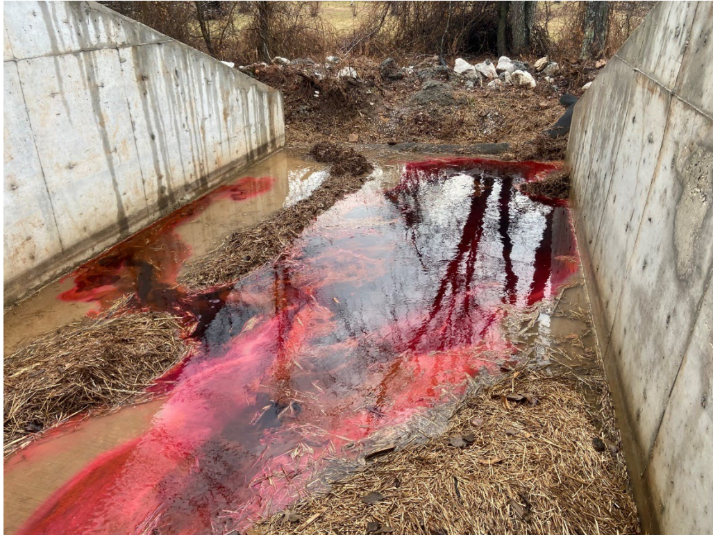
Figure 5. RWT dye introduced into the weir structure of a stormwater detention basin in the Northtown Park development.
