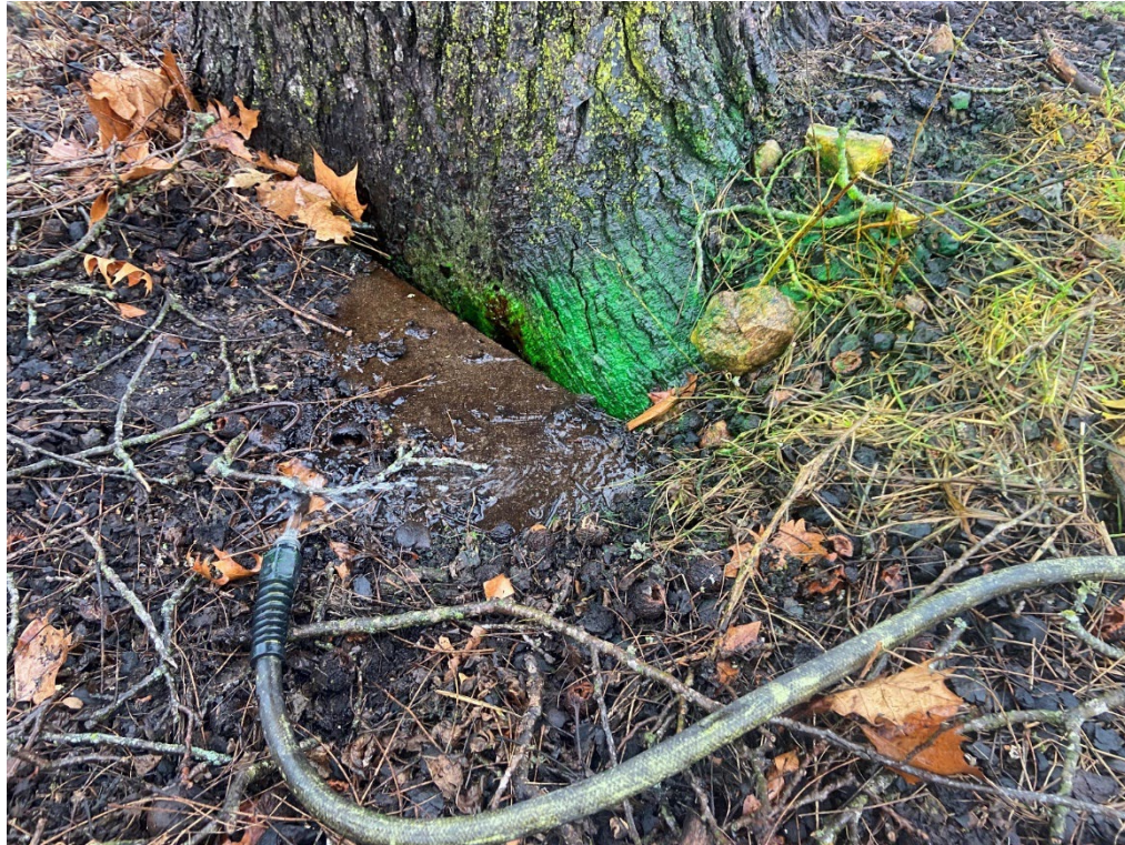
Figure 7. Flushing water behind Trace 23-02 with a garden hose. The small space between the tree and the slab covering the sinkhole allowed for the fluorescein introduction.
