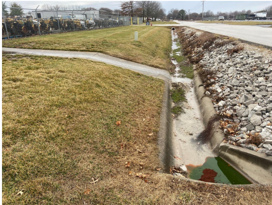
Figure 10. Eosine dye introduced into West Liberty Road culvert for Trace 23-04.
